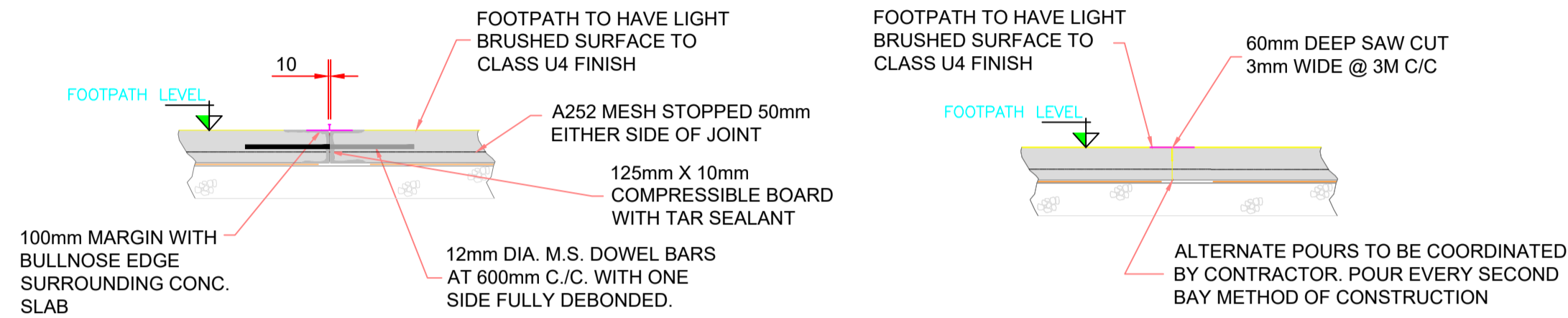
TYPICAL FOOTPATH CONTRACTION/CONSTRUCTION JOINT - MIN. 3M CTRS A1 SCALE 1:25
