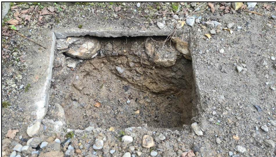
Plate 20 Test pit in SW of site
