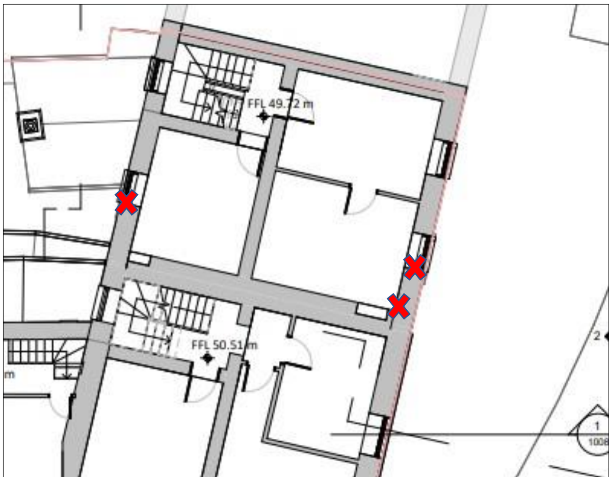
Figure 5. Highlights areas of damaged lintels on the second floor.
