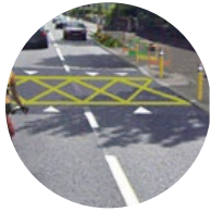
Raised pedestrian crossing
