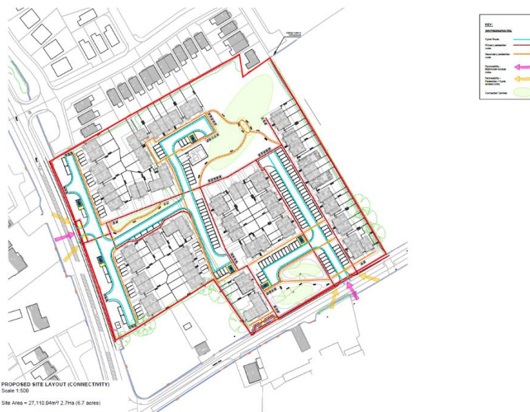
Extract of drawing N°210503-03-014, Connectivity. It shows road's layout and connectivity alternatives.
