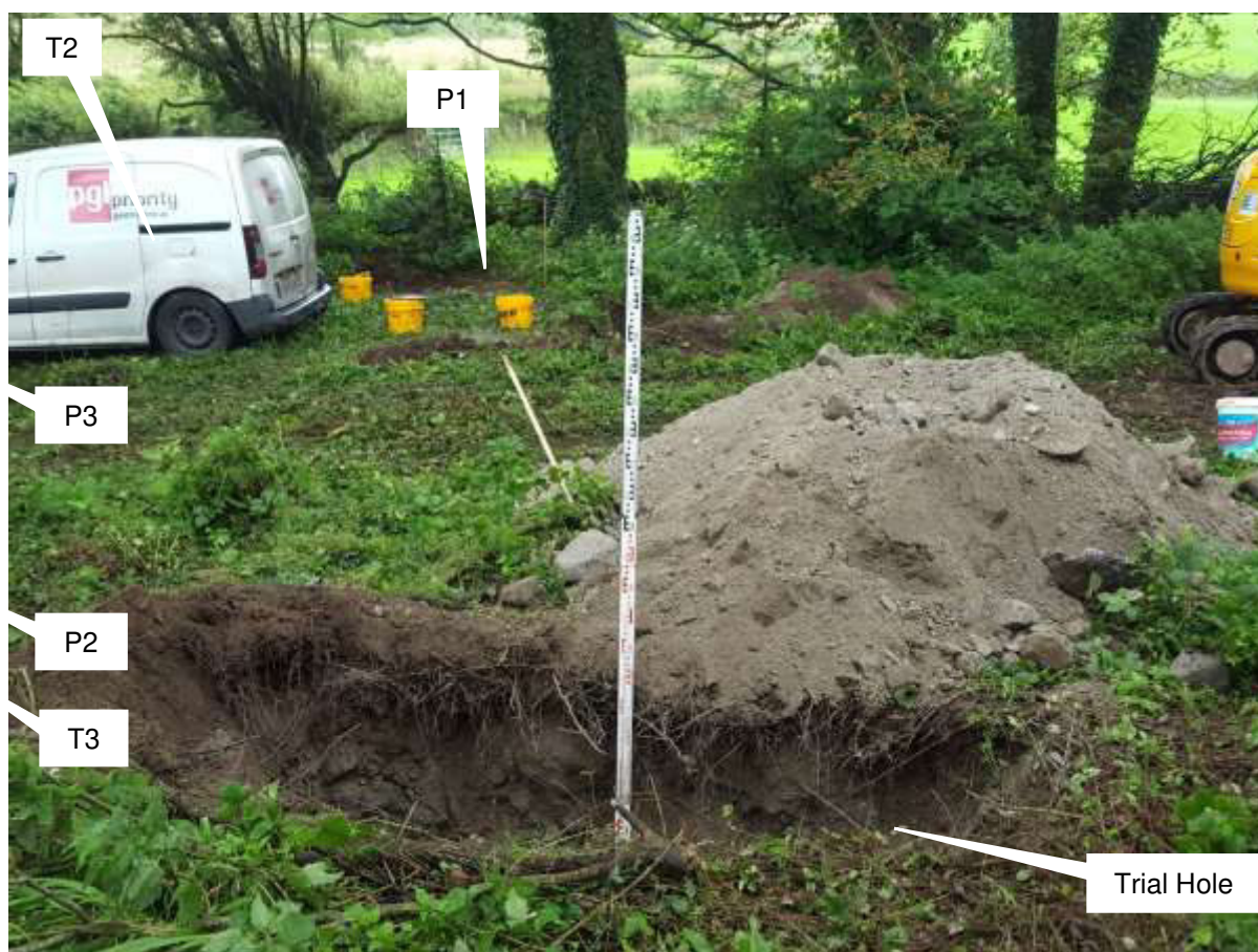
Overview of percolation test area, showing Trial Pit, T & P test holes.
