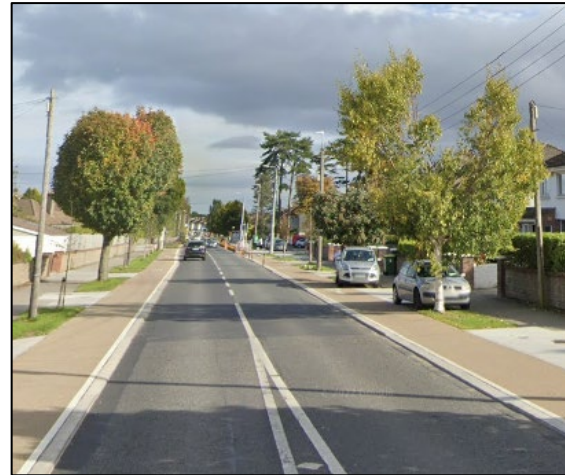
Figure 5-2: Example of a Segregated Cycle Track
