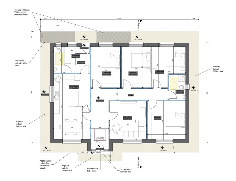
Ground Floor Plan Area: 134.60m<sup>2</sup> Scale 1:100
