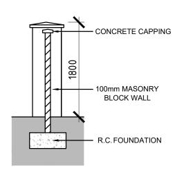
SECTION THROUGH WALL "C" SCALE 1:50
