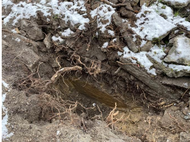
Photograph 3: Note the filled ground and debris overlying the solid layer at 1.3m below existing ground level
