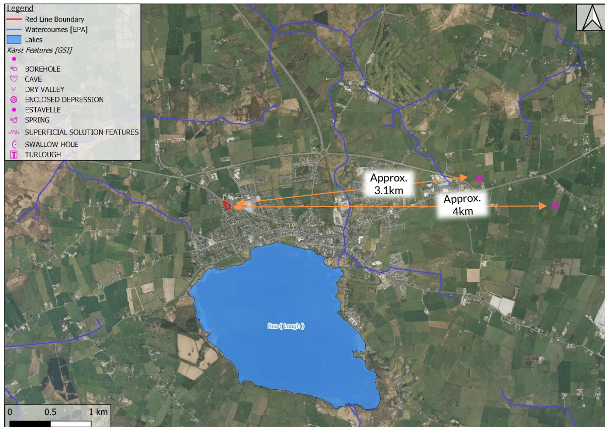
Figure 3-4 GSI Mapping of Karst Features
