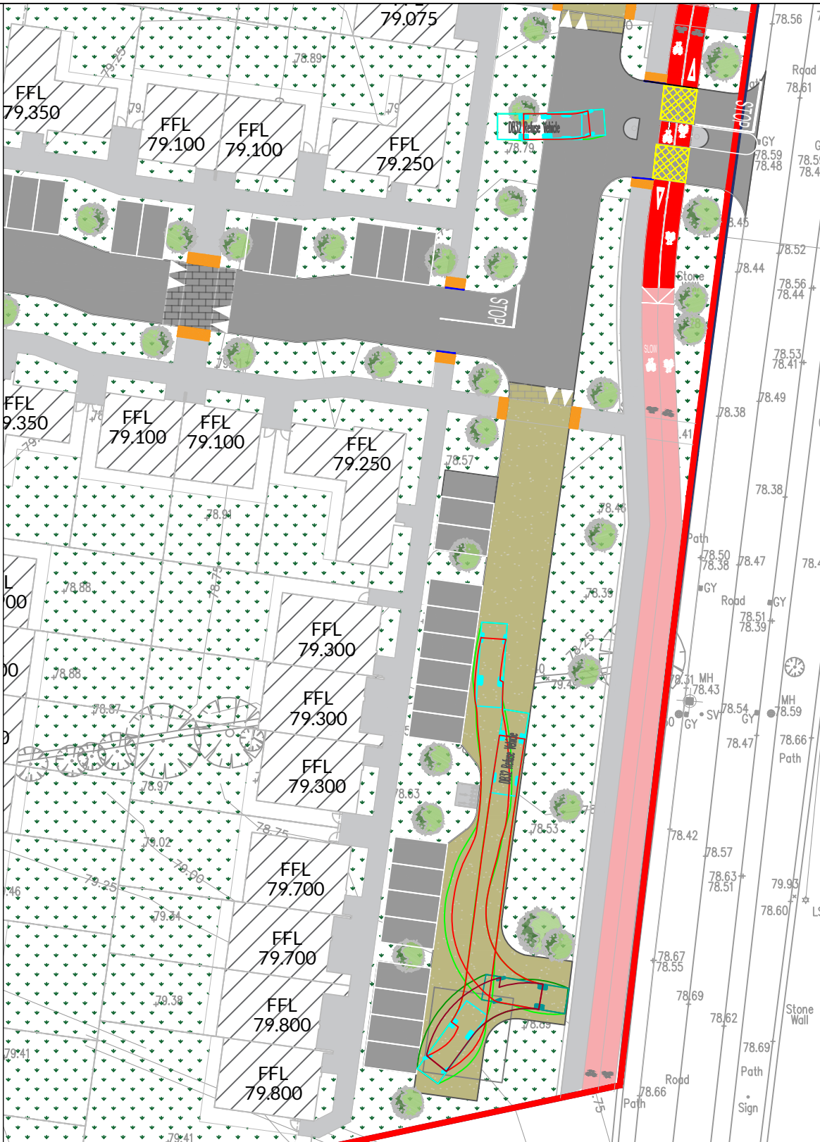
SWEPT PATH ANALYSIS - REFUSE VEHICLE SCALE 1:500
