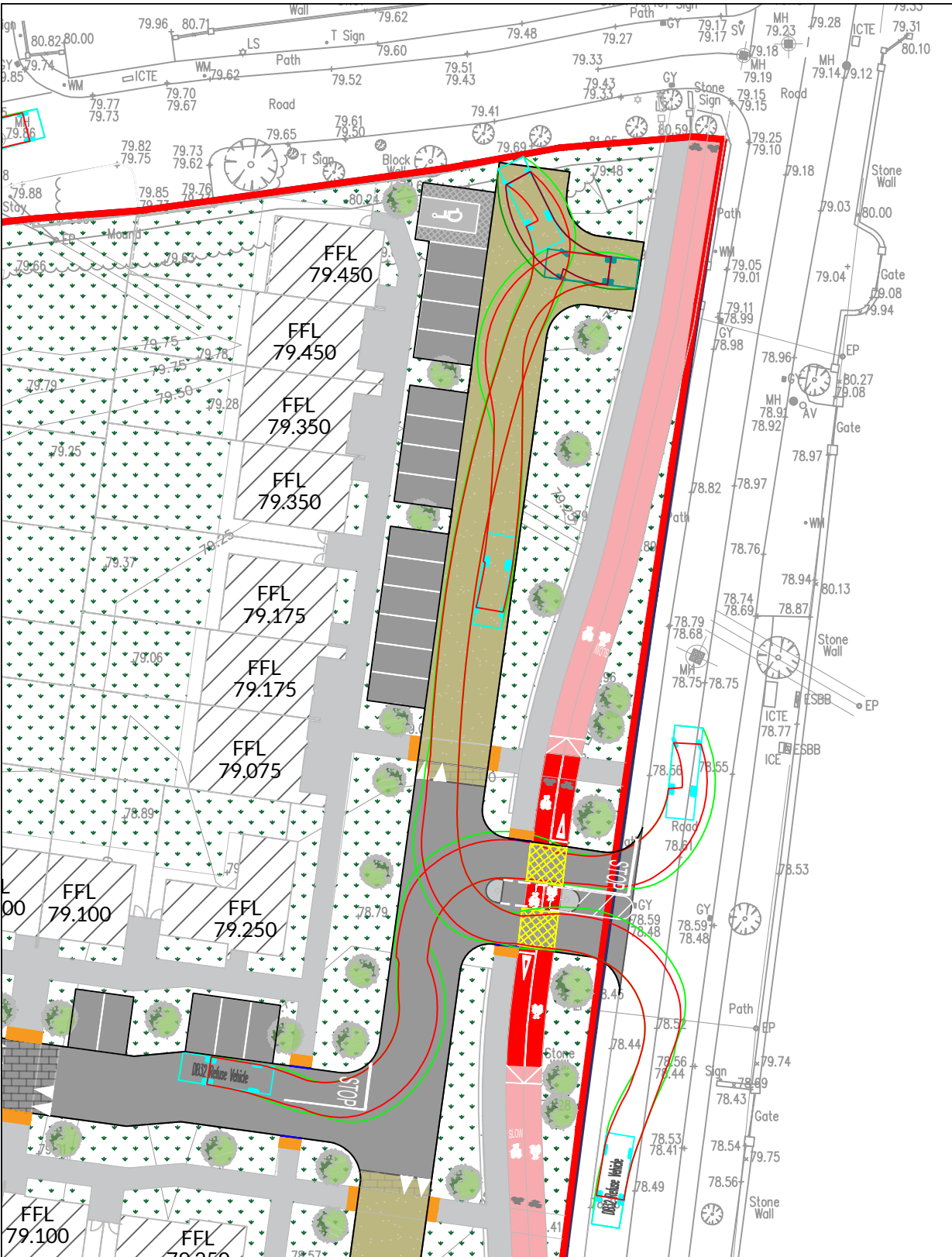
SWEPT PATH ANALYSIS - REFUSE VEHICLE SCALE 1:500
