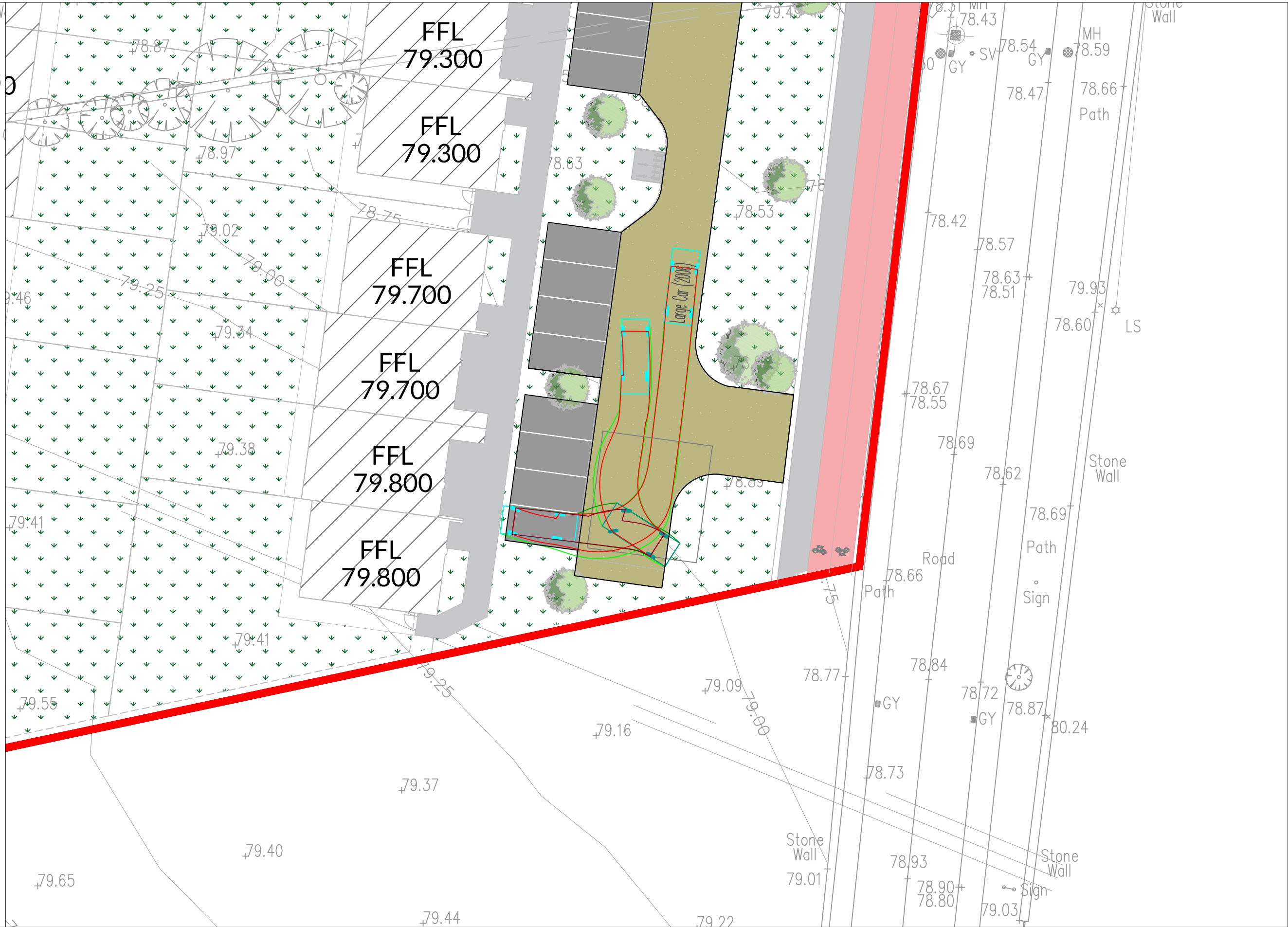
SWEPT PATH ANALYSIS - LARGE CAR SCALE 1:500
