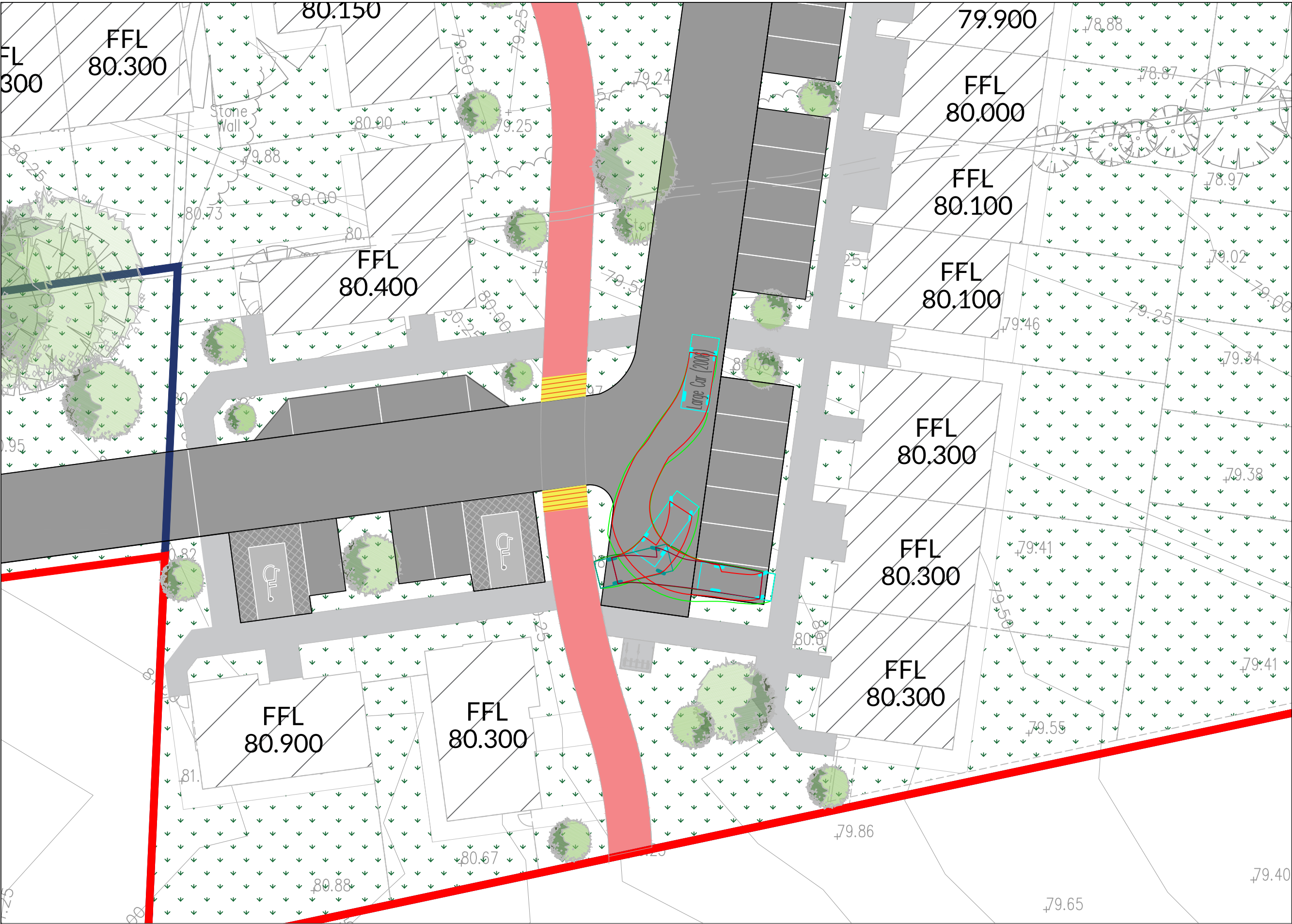
SWEPT PATH ANALYSIS - LARGE CAR SCALE 1:500
