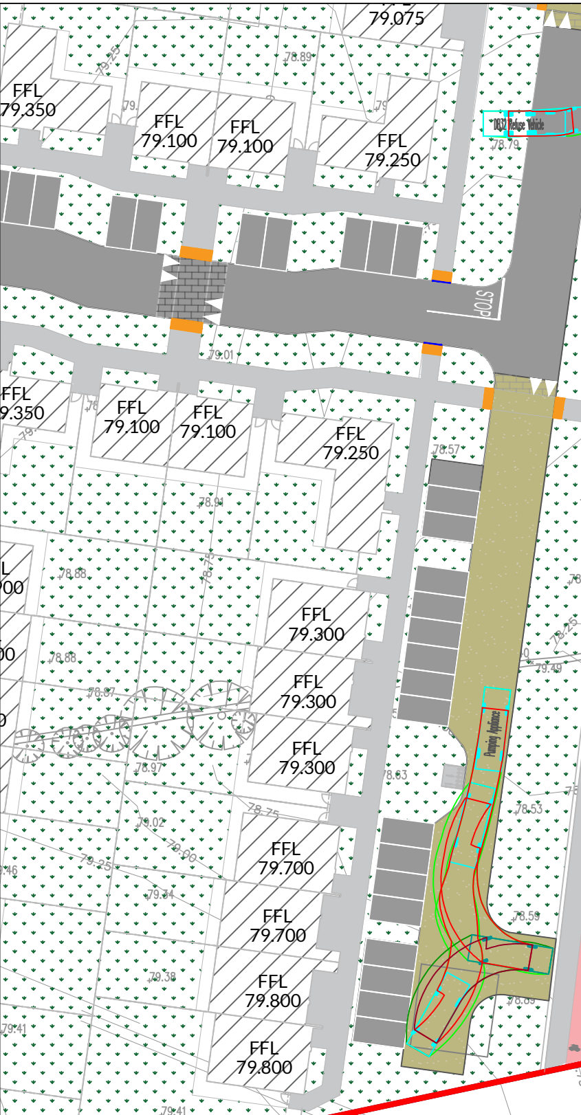
SWEPT PATH ANALYSIS - FIRE TENDER SCALE 1:500
