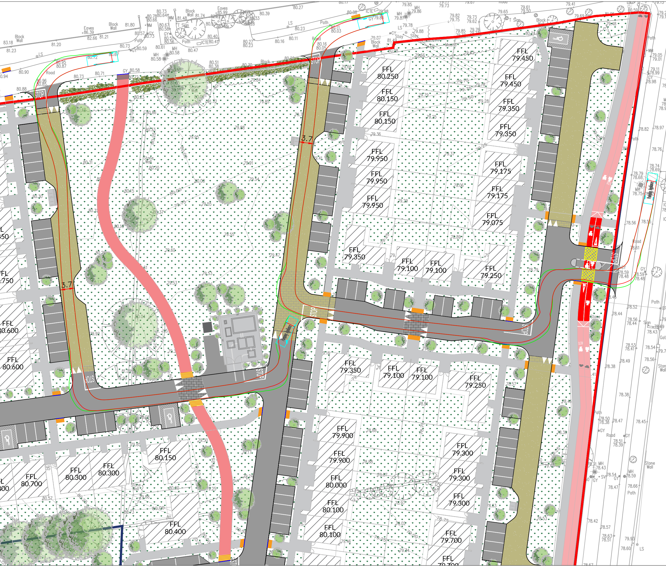
SWEPT PATH ANALYSIS - FIRE TENDER SCALE 1:500
