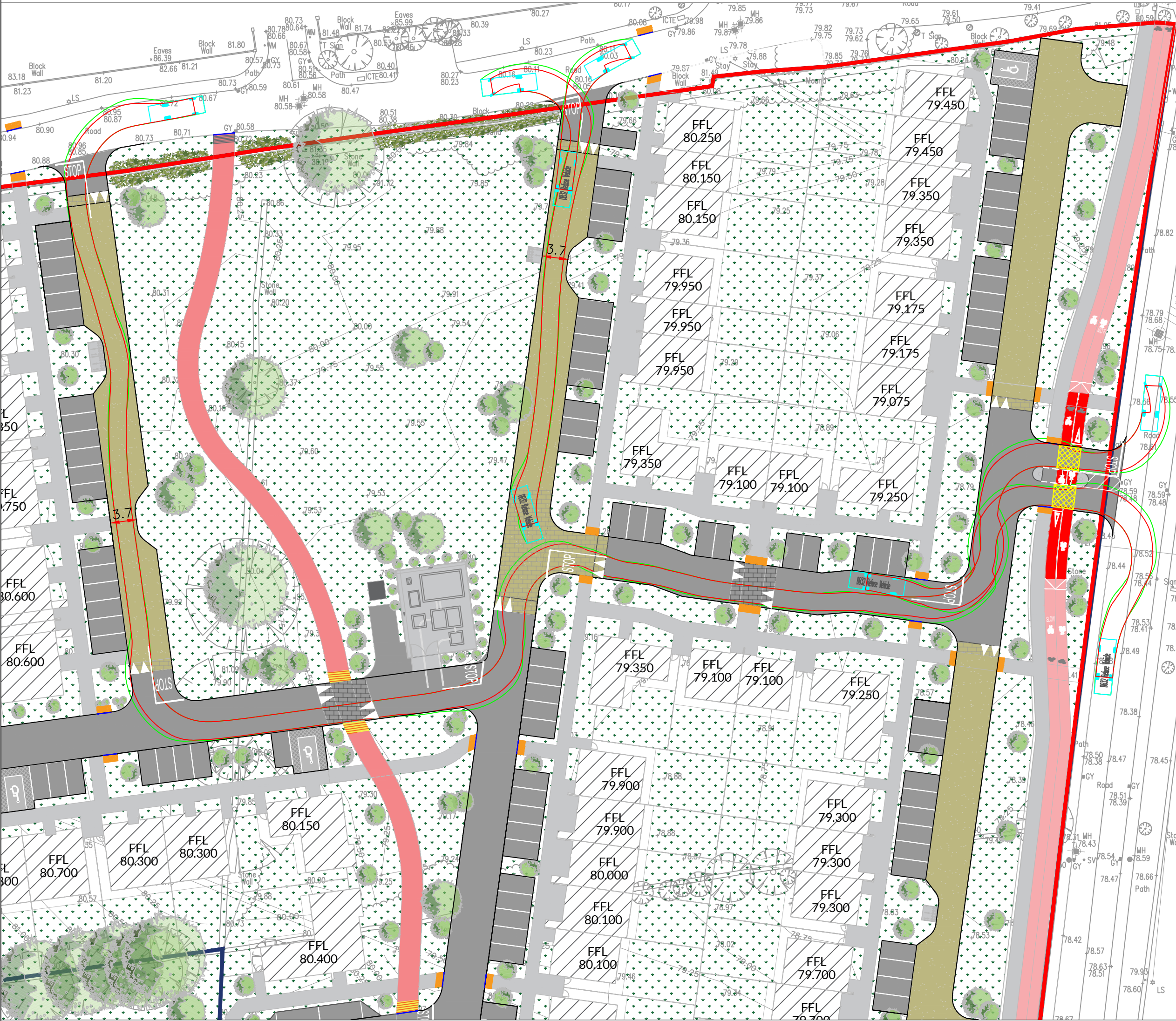
SWEPT PATH ANALYSIS - REFUSE VEHICLE SCALE 1:500
