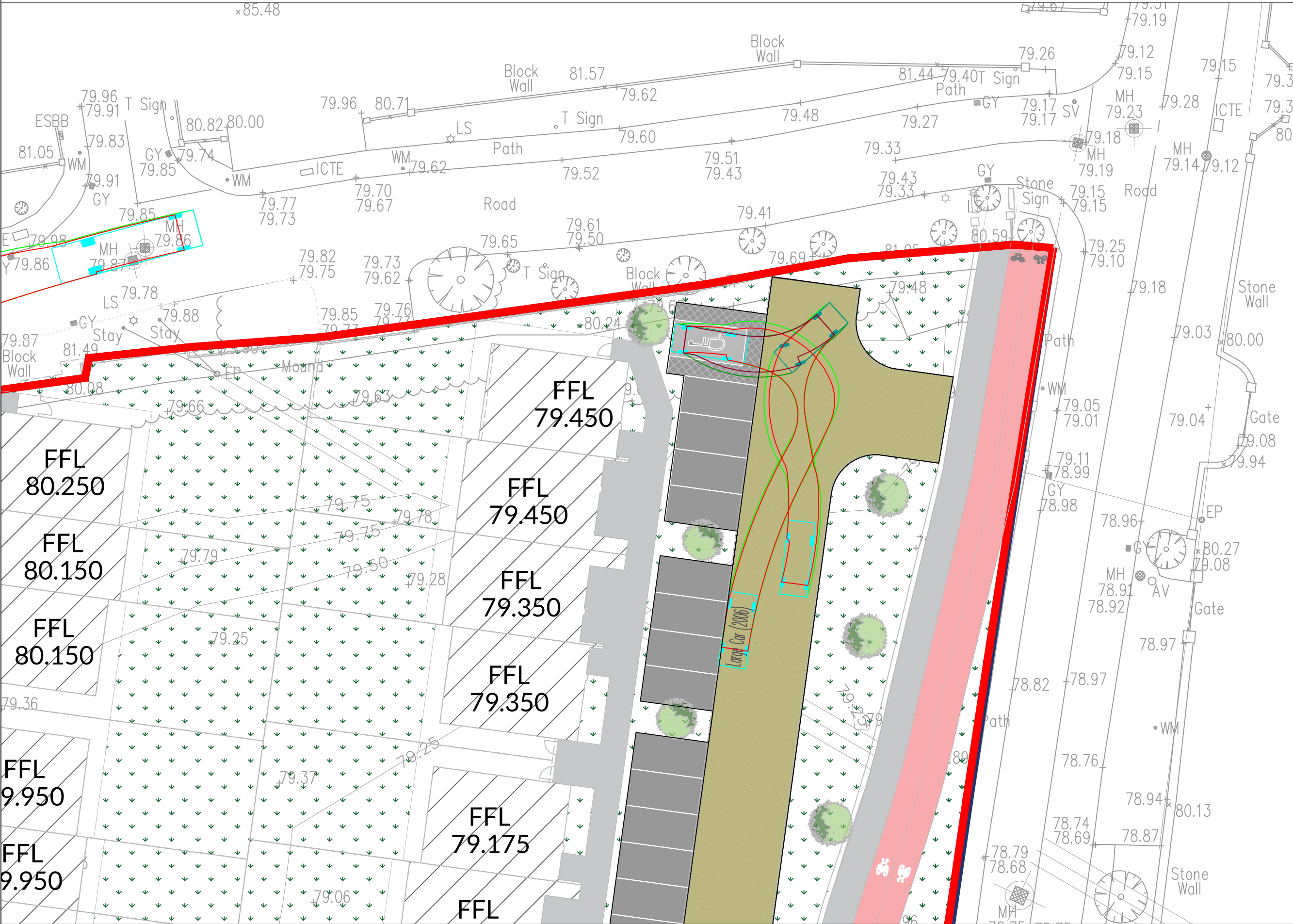
SWEPT PATH ANALYSIS - LARGE CAR SCALE 1:500
