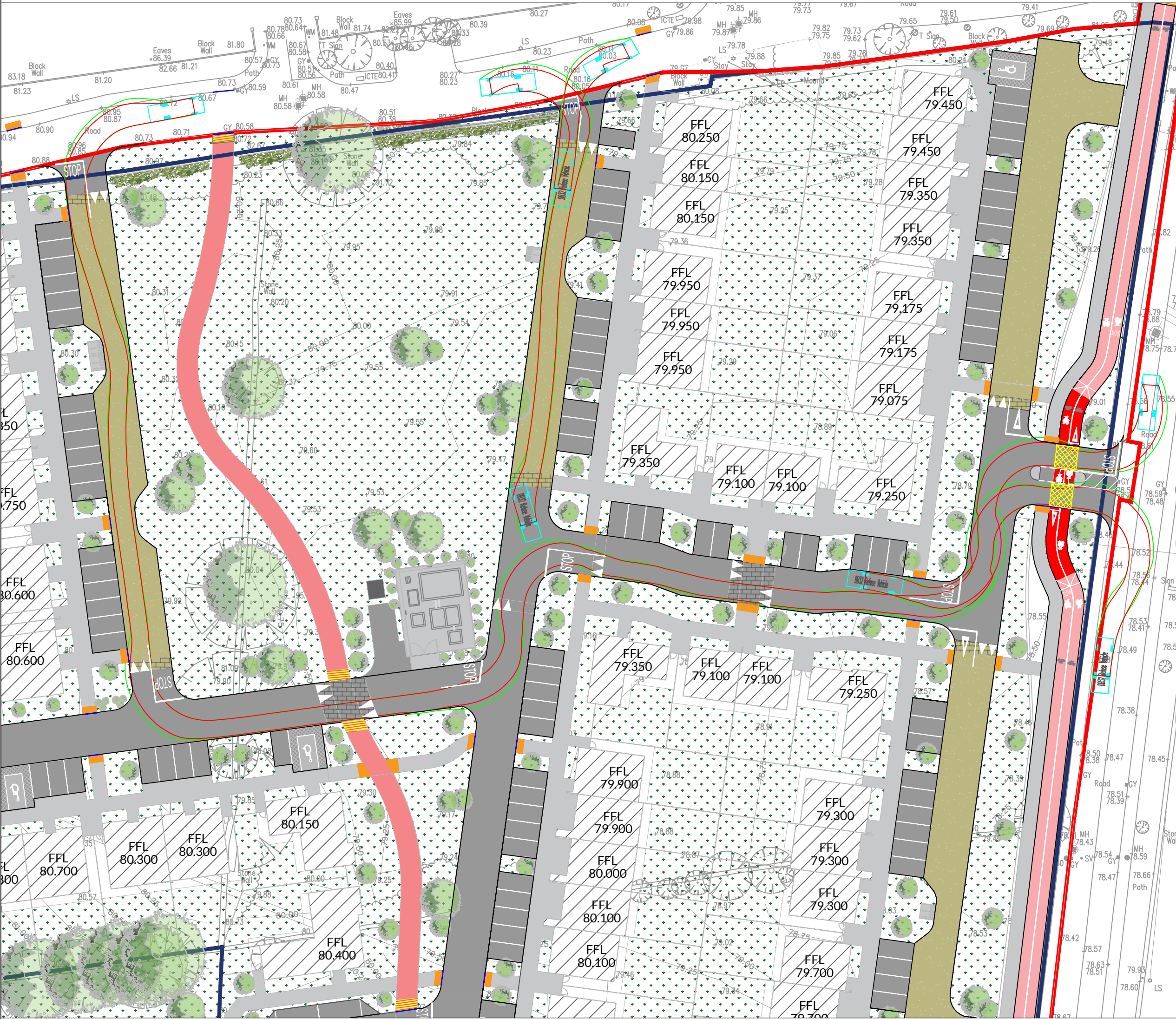
SWEPT PATH ANALYSIS - REFUSE VEHICLE SCALE 1:500
