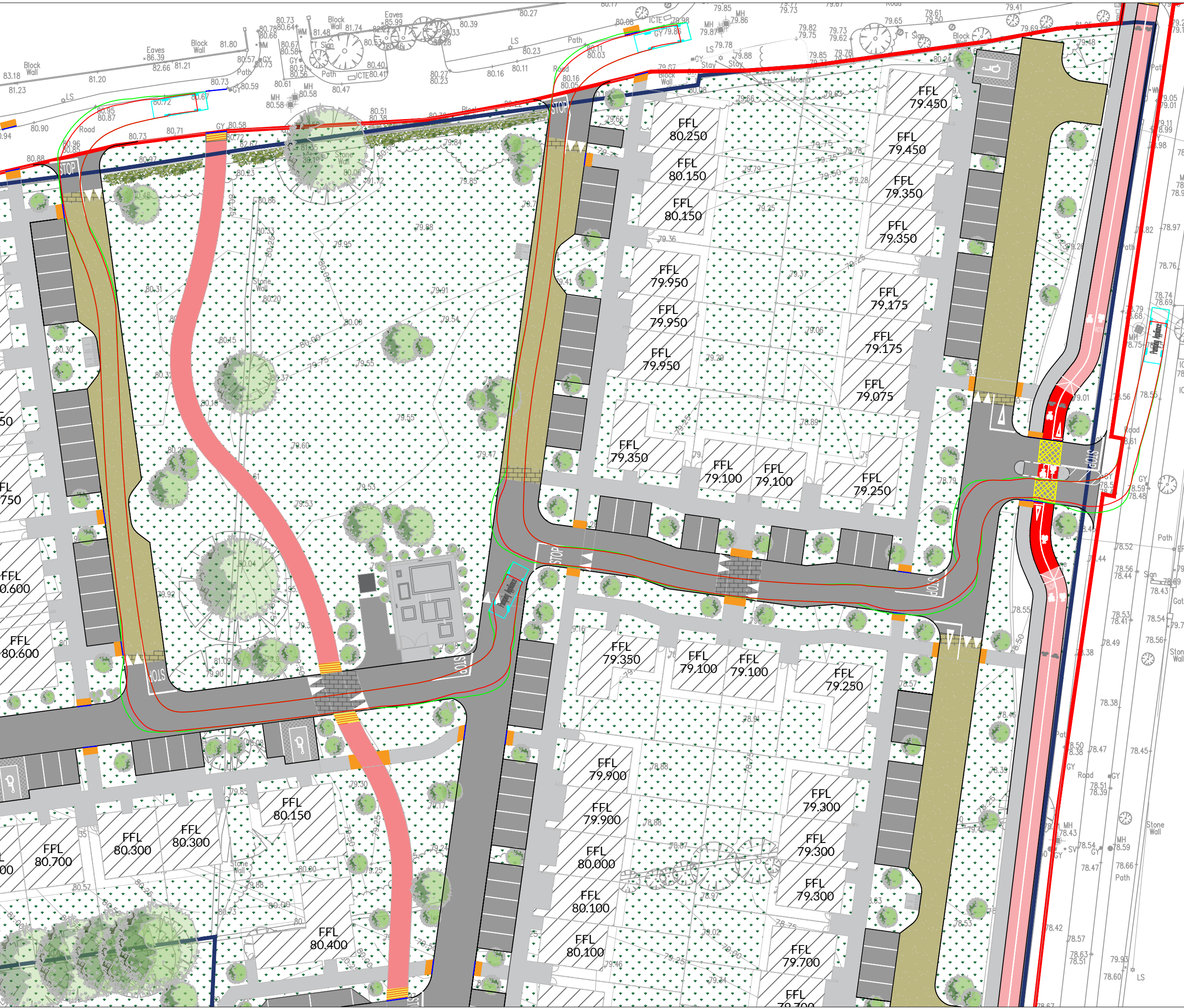
SWEPT PATH ANALYSIS - FIRE TENDER SCALE 1:500
