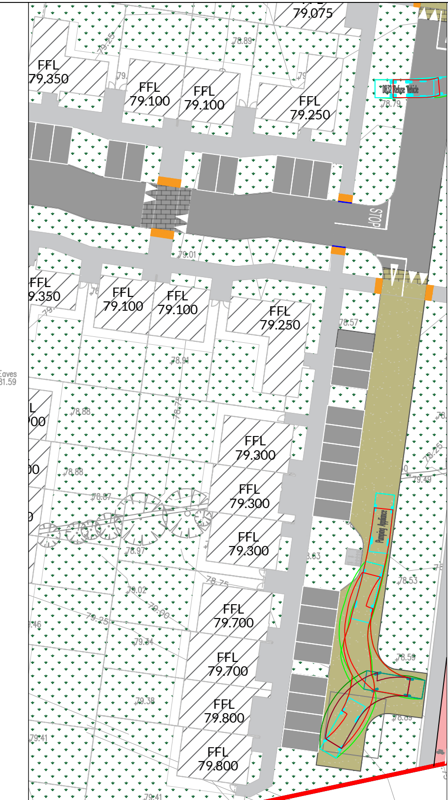
SWEPT PATH ANALYSIS - FIRE TENDER SCALE 1:500
