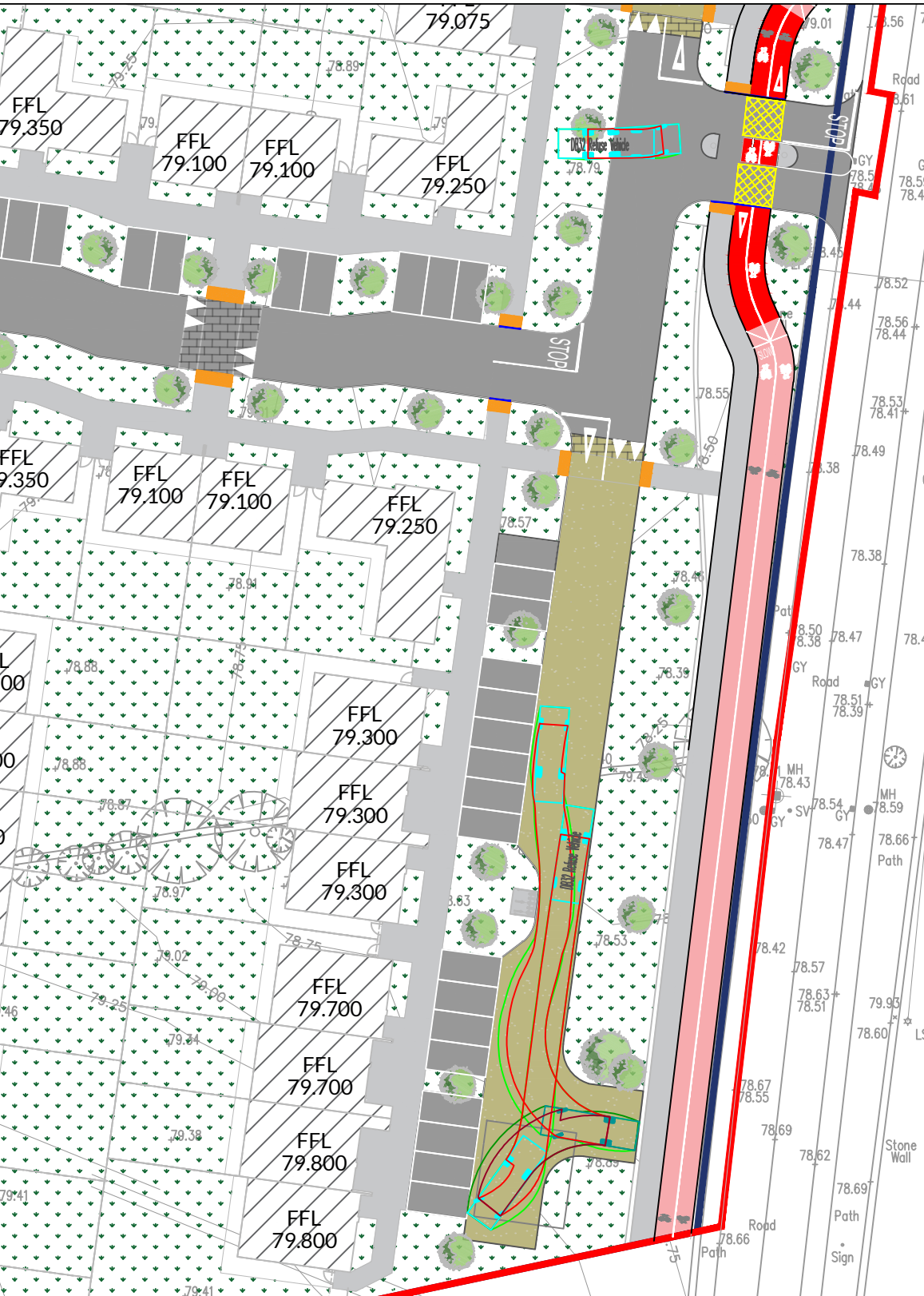
SWEPT PATH ANALYSIS - REFUSE VEHICLE SCALE 1:500
