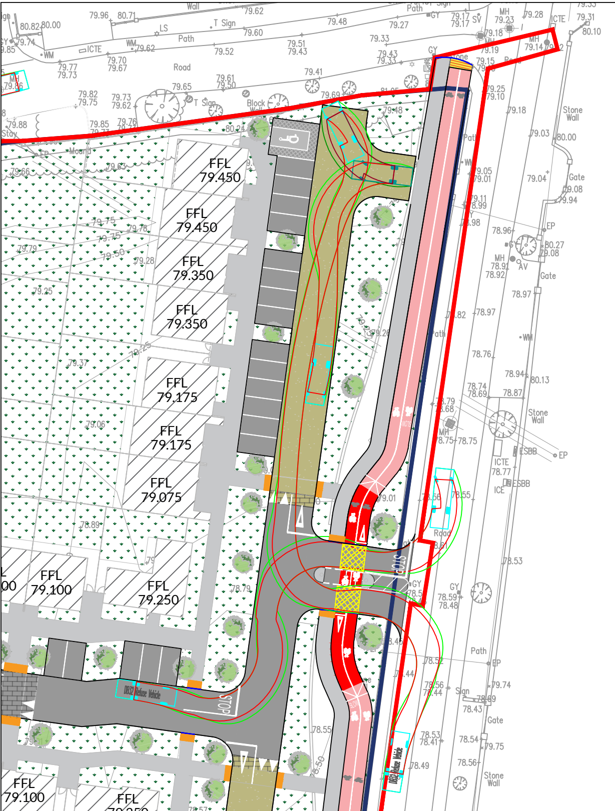
SWEPT PATH ANALYSIS - REFUSE VEHICLE SCALE 1:500
