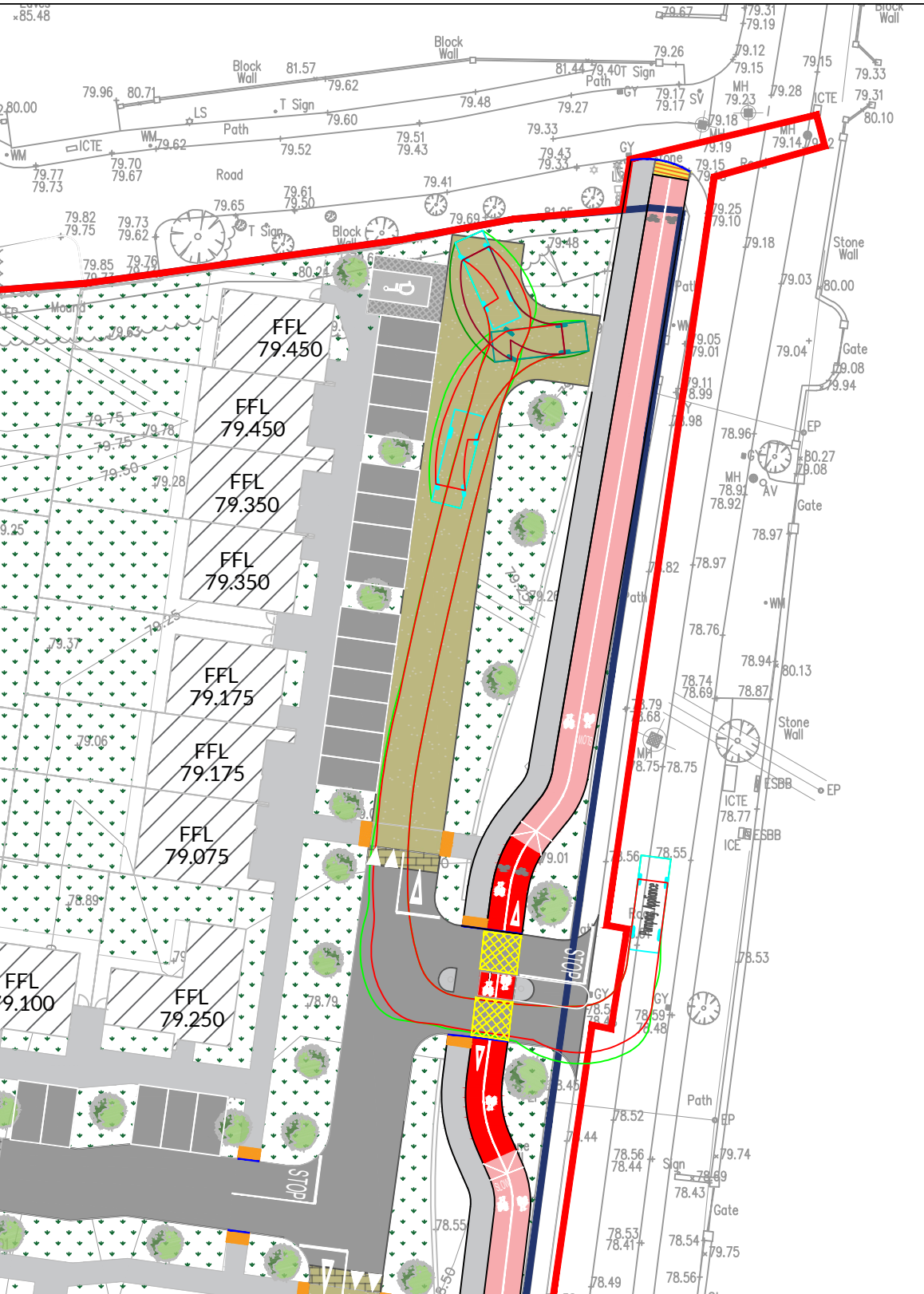
SWEPT PATH ANALYSIS - FIRE TENDER SCALE 1:500
