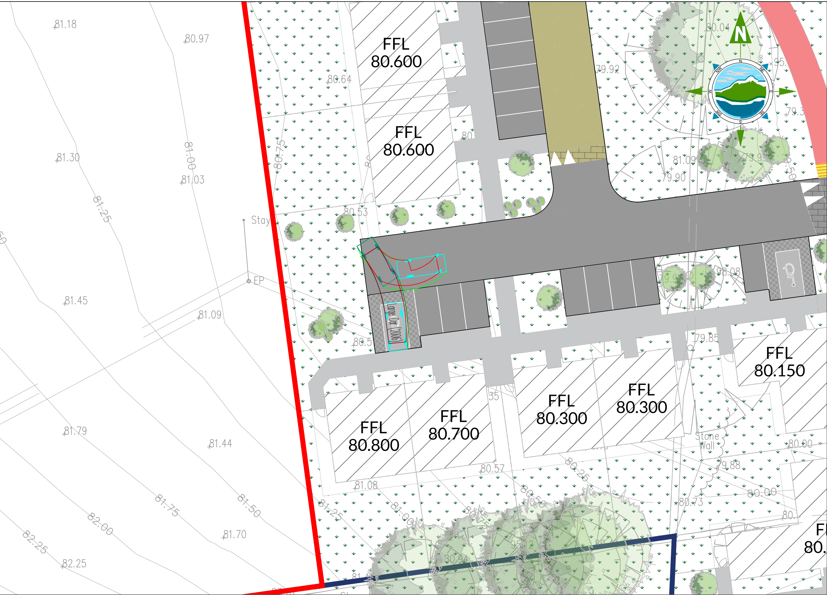
SWEPT PATH ANALYSIS - LARGE CAR SCALE 1:500
