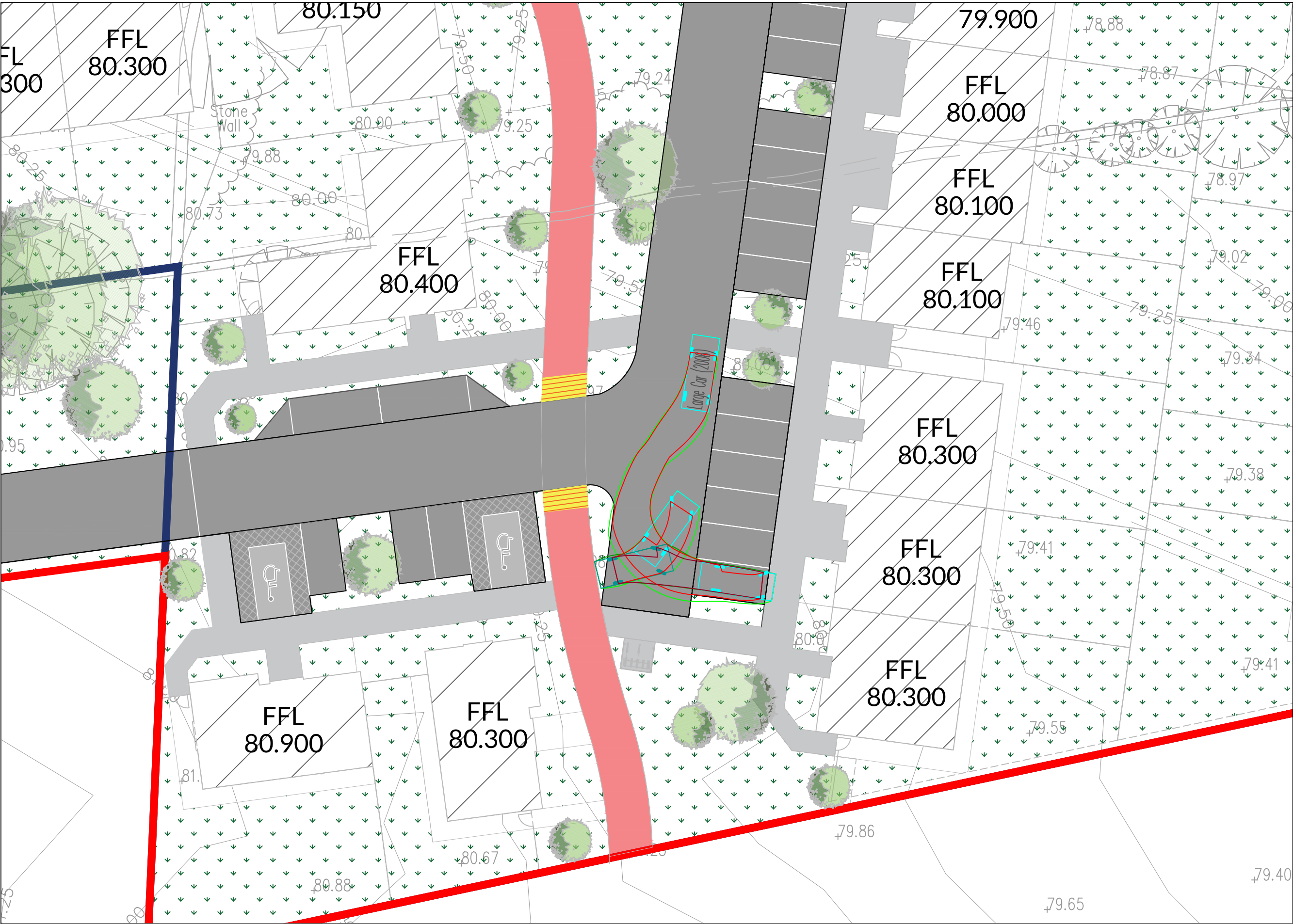
SWEPT PATH ANALYSIS - LARGE CAR SCALE 1:500
