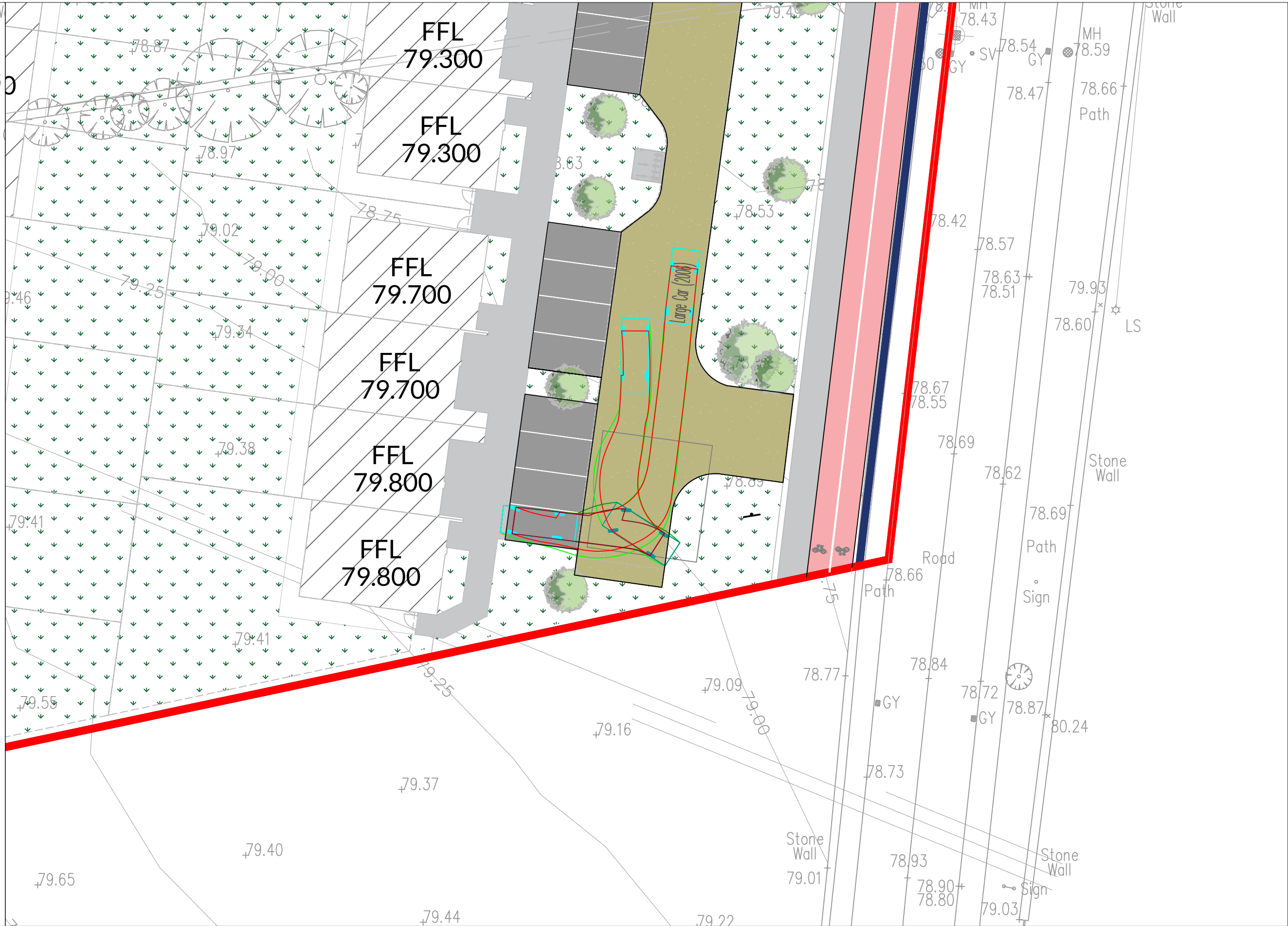
SWEPT PATH ANALYSIS - LARGE CAR SCALE 1:500
