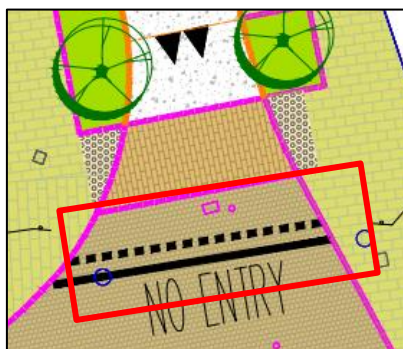
Figure 2-16 No Entry Road marking (Dwg No. 11623_LD_HL_TC_003)
