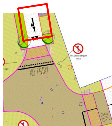
Figure 2-17 Left turn road marking not included on the design (Dwg No. 11623_LD_HL_TC_001)
