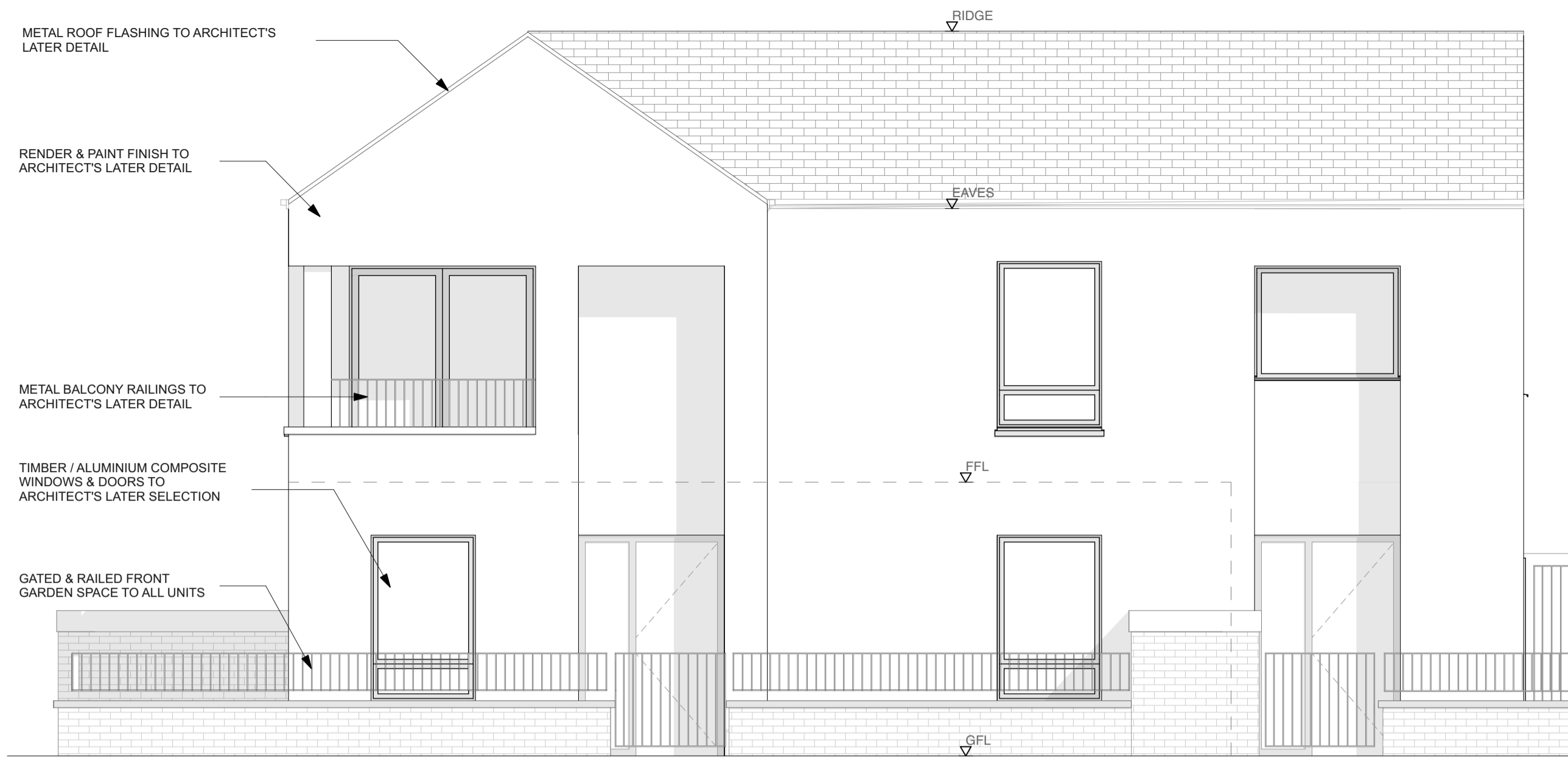
UNIT TYPE A/B - FRONT ELEVATION 1 1:50
