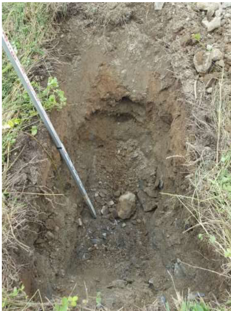
Trial Pit dug to 1.6m deep 29-06-2020.
