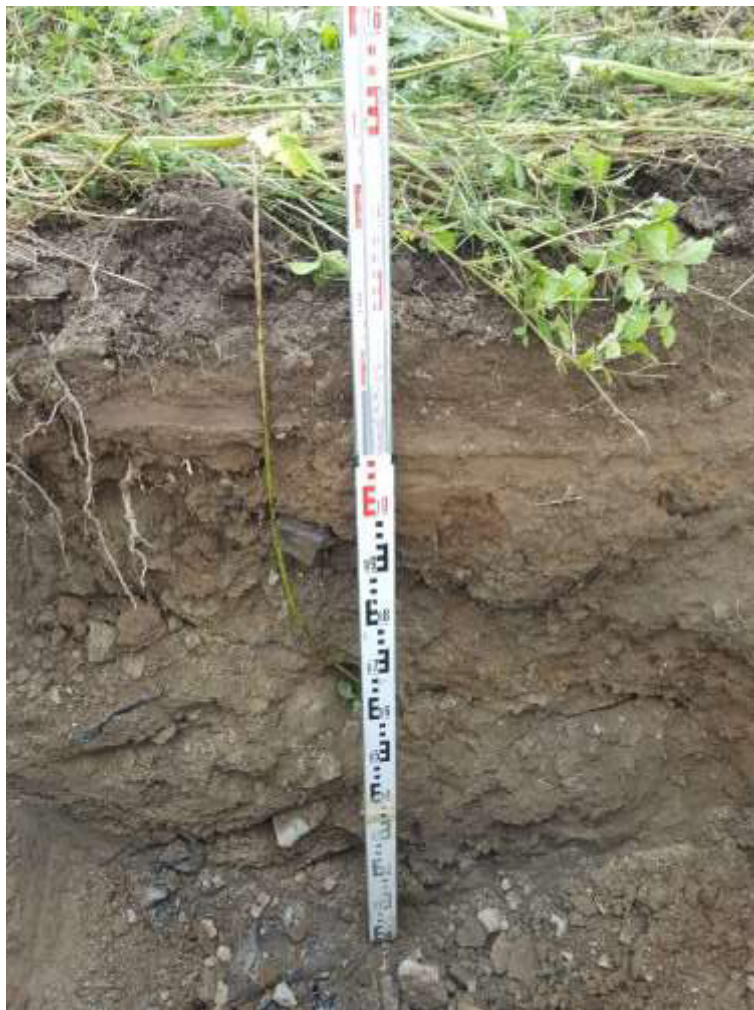
Trial Pit dug to 1.6m deep 29-06-2020.
