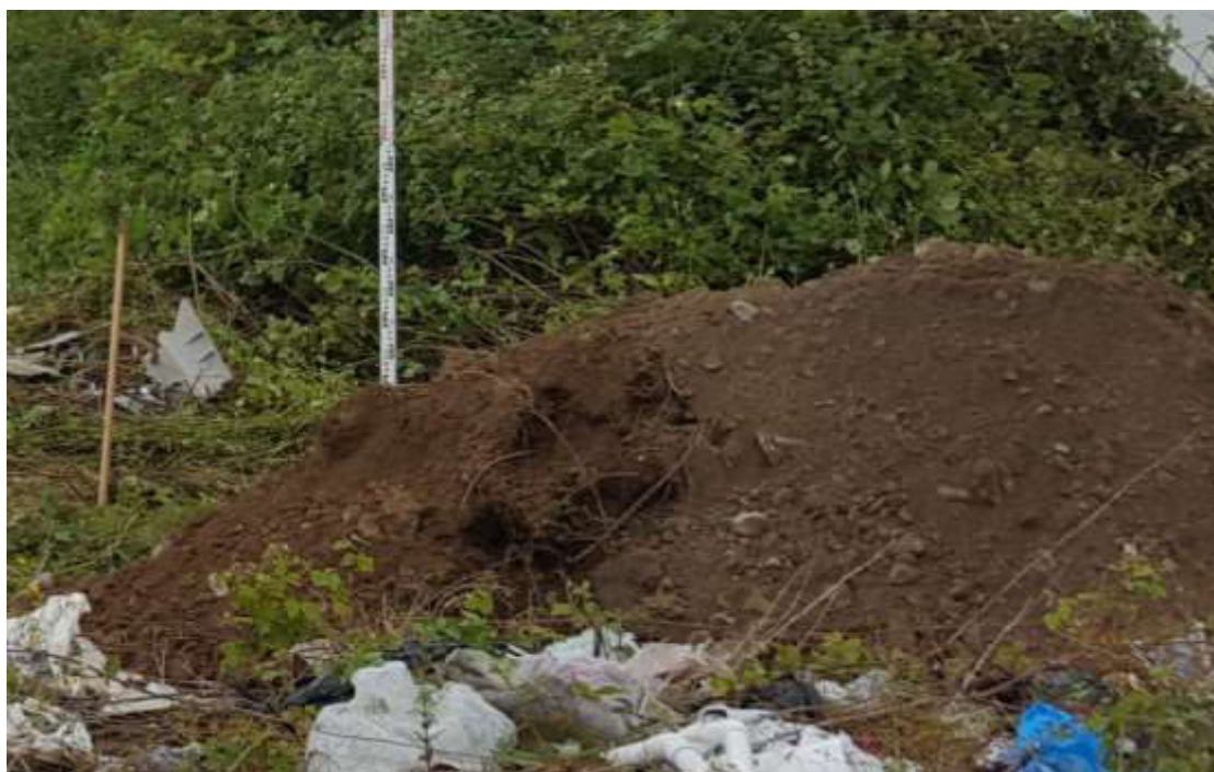
Trial Pit Spoil, pit dug to 1.9m deep 01-07-2020.
