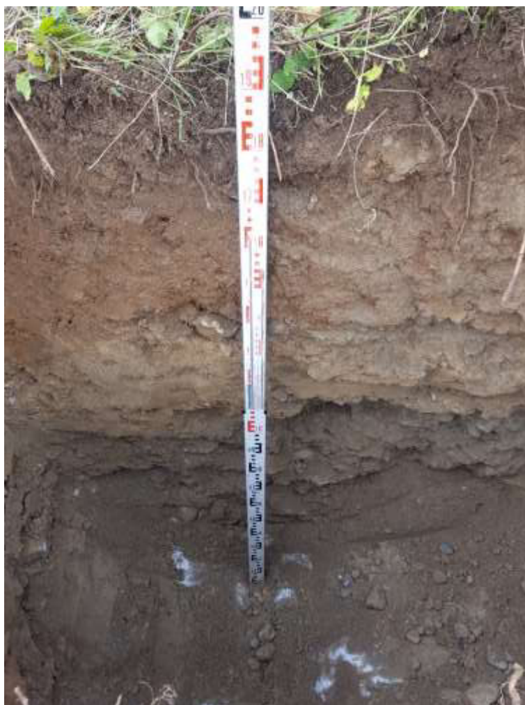
Trial Pit dug to 1.9m deep 01-07-2020.
