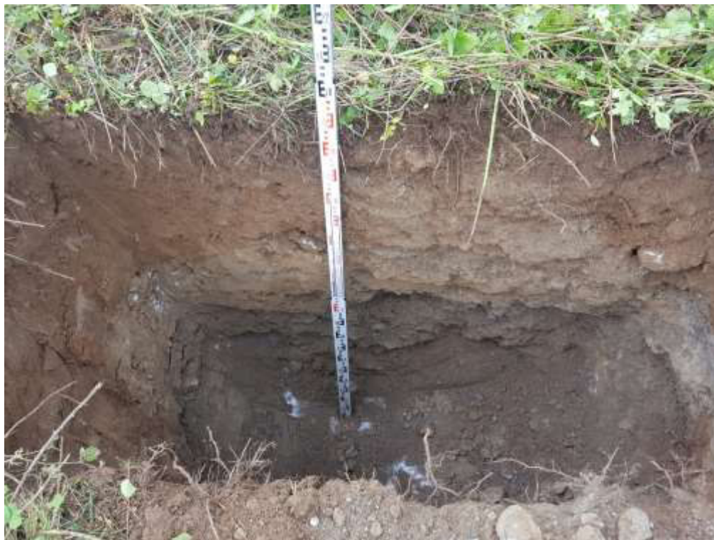
Trial Pit dug to 1.9m deep 01-07-2020.
