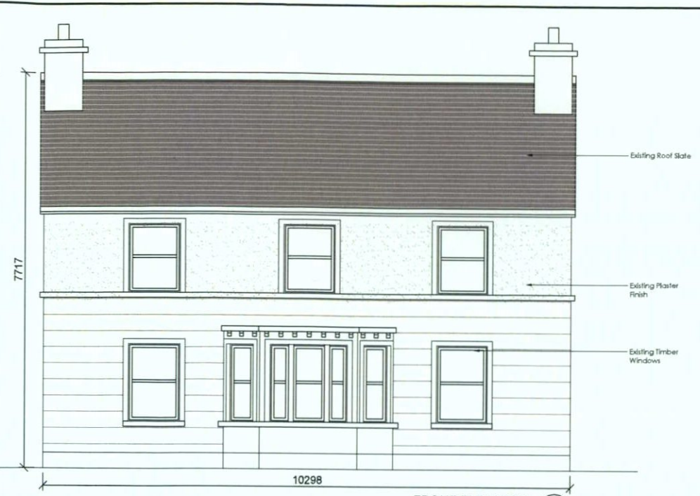
FRONT ELEVATION Scale 1:50
