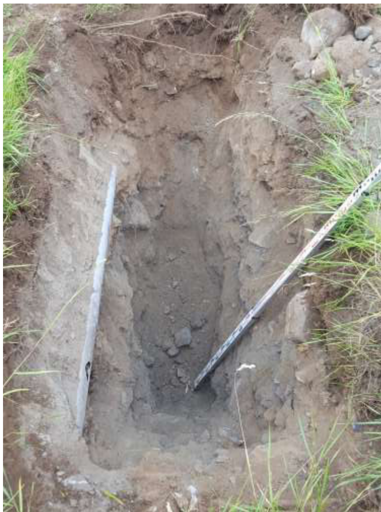
Trial Pit dug to 1.95m deep 29-06-2020.
