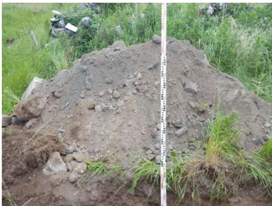
Trial Pit Spoil, Pit dug to 1.95m deep 29-06-2020.
