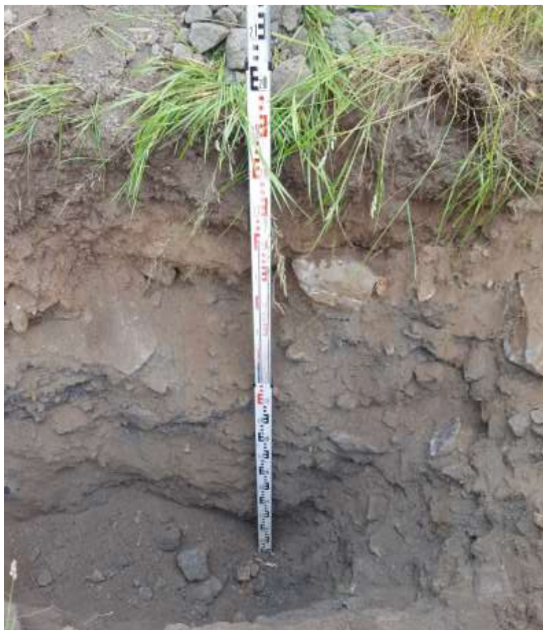
Trial Pit dug to 1.95m deep 29-06-2020.
