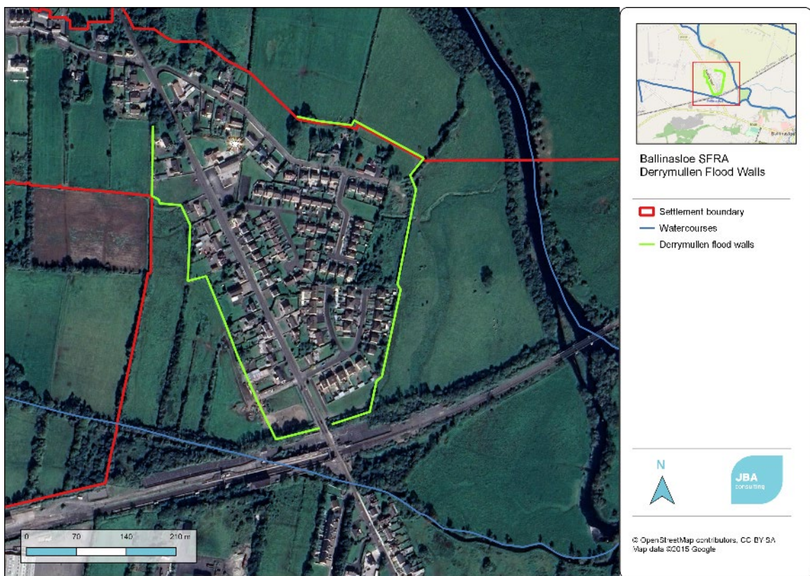
Figure 4-2 Derrymullan Flood Wall
