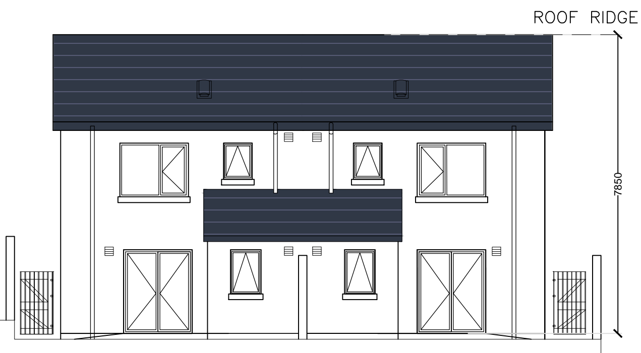
REAR ELEVATION UNITS 3,4,5,& 6
