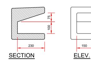
DETAILS OF TOE HOLD SCALE 1:10
