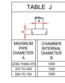
MANHOLE TYPE J 1m < DEPTH TO CROWN < 3m
