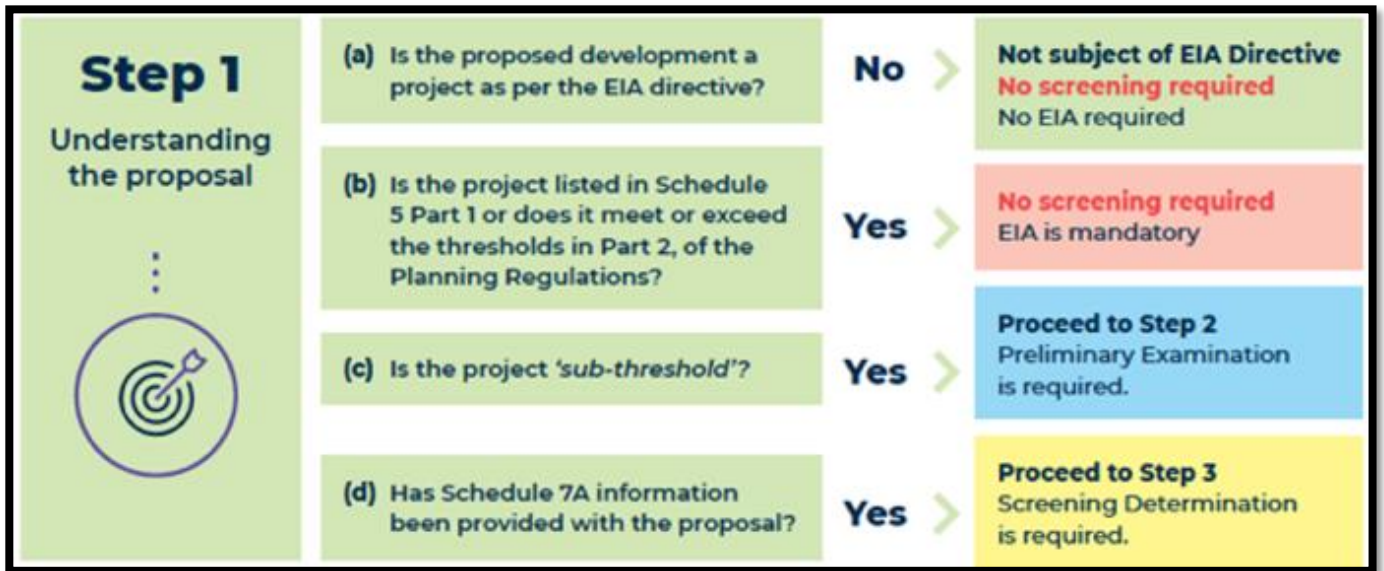
Figure 5: Extract from OPR Guidance showing Step 1 of “Step-by-step approach to EIA Screening for Development Proposals.”
