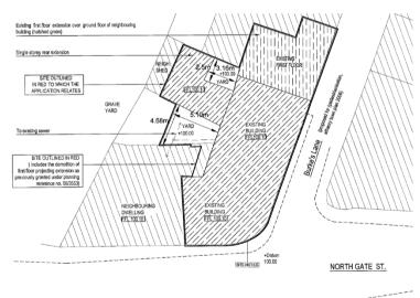
The current site consists of a two-storey block built structure with a slate roof facing onto North Gate Street and Burkes Lane with a single storey extension constructed to the to the Northeast and adjoining the main structure and creating two small yards.
