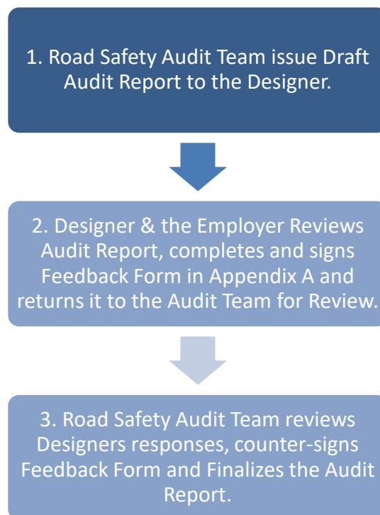
Figure 5.1 – Road Safety Audit Sign-Off and Completion Process
