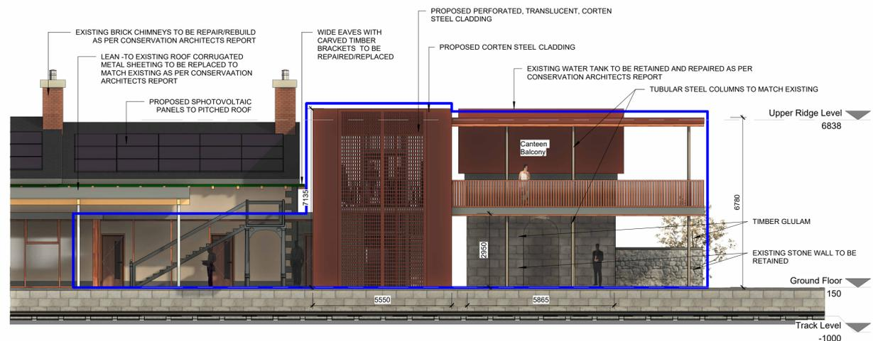
26 South-West (Part Elevation to Platform) Elevation- Proposed
