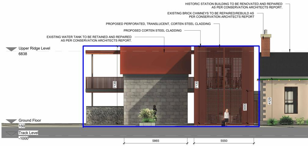
21 North-East Elevation(Part Elevation to Sean Purcell Road) - Proposed
