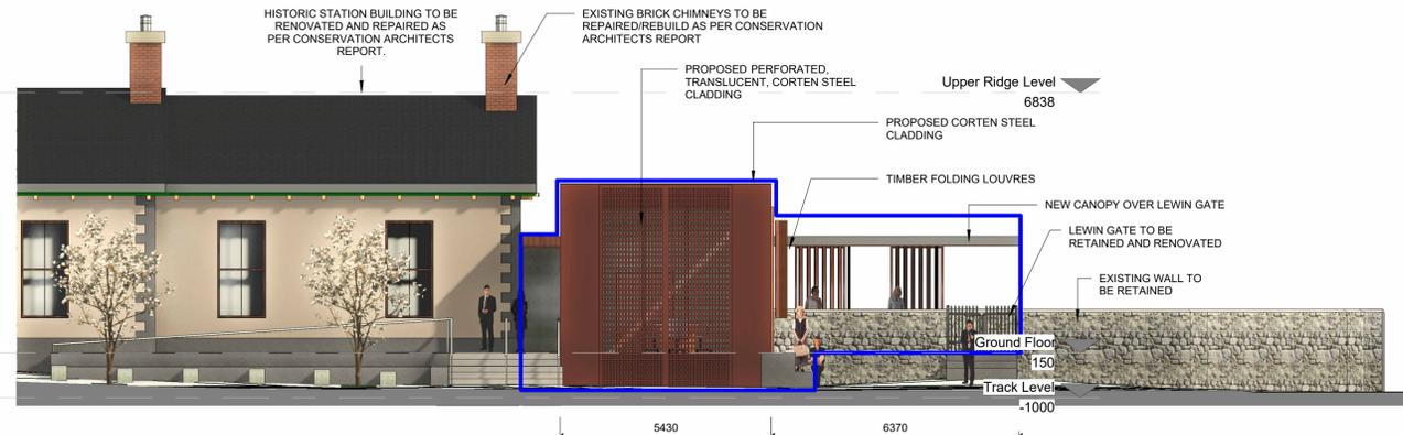
22 North-East Elevation(Part Elevation to Sean Purcell Road) - Proposed
