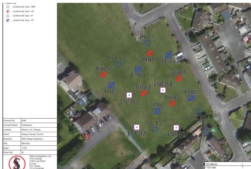
Figure 4.1 Site investigation locations (Source: Site Investigations Ireland LTD)
