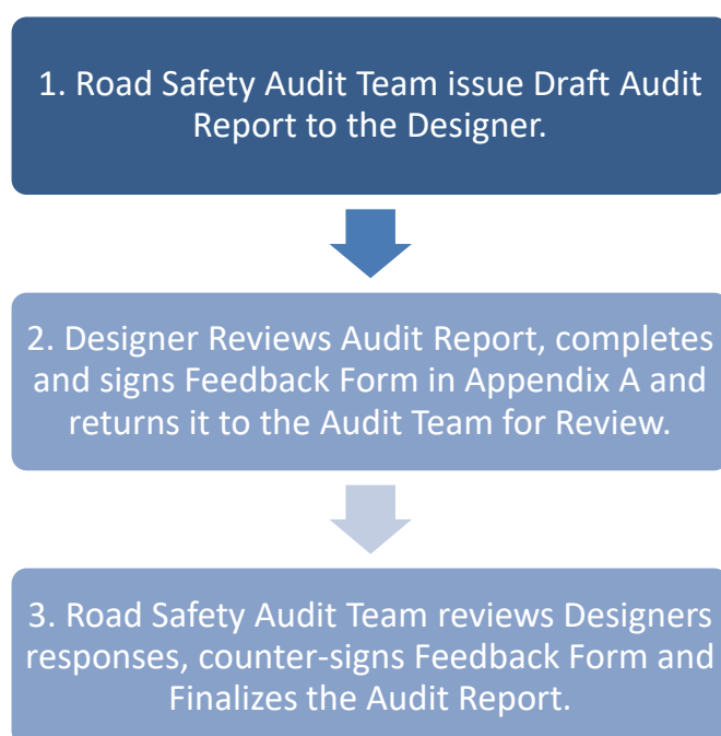
Figure 4.1 – Road Safety Audit Sign-Off and Completion Process
