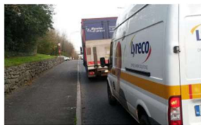
Figure: Photograph showing the impact that using a 3.2m traffic lane on an arterial road has on road space for people on bicycles. Location: Tuam Road, Galway.
