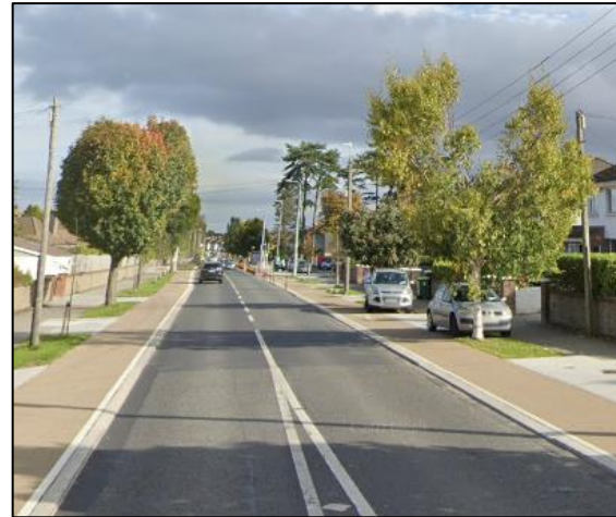
Figure 5-2: Example of a Segregated Cycle Track
